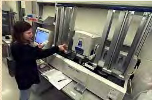
The PlateMate Plus robot transfers colonies from 384-well stock plates to new 384-well plates for lysing.
