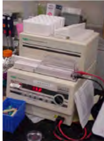
An electroporation machine: induces bacteria to open their pores with an electric shock
