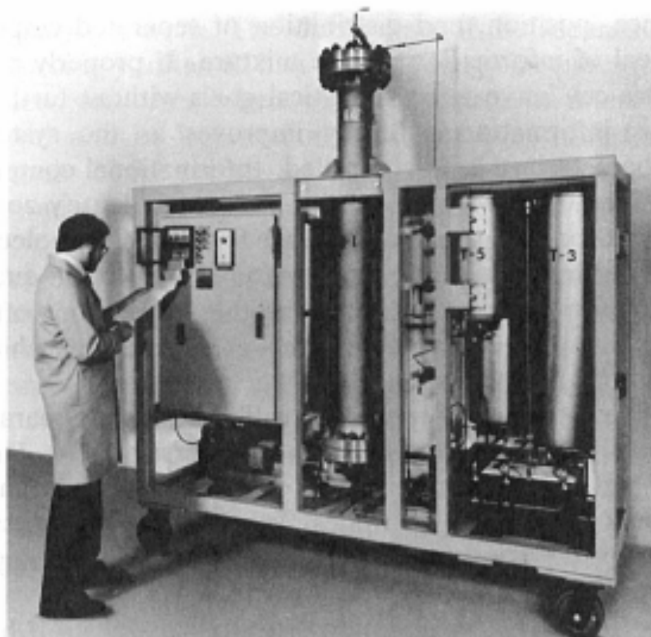
Figure 1.2. Preparative scale liquid chromatography unit with 6 ft (1.8 m) long column (in center) having an inner diameter of 6 in (15 cm). Up to 2 L of sample solution can be injected and processed in a single 90-min run. (Courtesy Thomas J. Filipi and Whatman Chemical Separation Division.)
