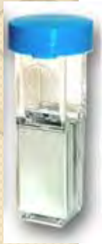
A cuvette for use in the electroporation machine
