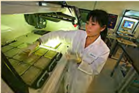
A technician loads plates into the colony picking machine.
