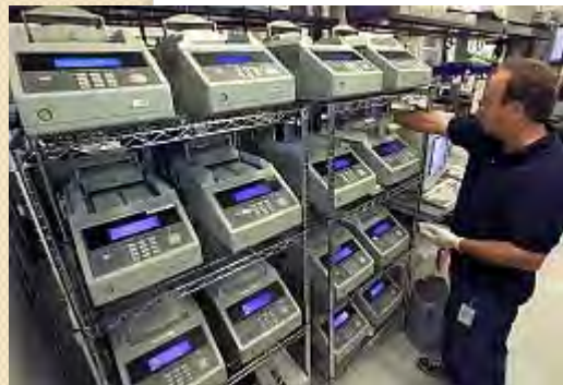
Thermal cyclers heat up bacterial cells to break them open.
